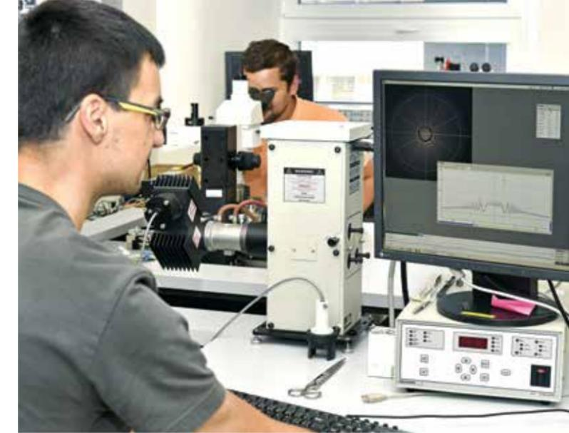
"Currently, we are examining the way temperature affects a lubricated contact so we use an infrared camera to observe the reaction of lubricants during the slip of friction parts, when surfaces move at different speeds," described Křupka
