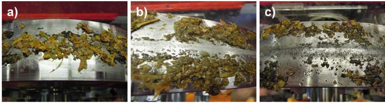
Fig. 13. Photographs of disc surface during test with leaf mixture (a) before the test; (b) after run in; (c) after sanding.
