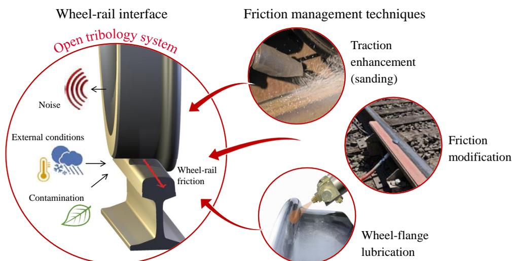
Fig. 10 Wheel-rail interface and relevant friction management techniques
