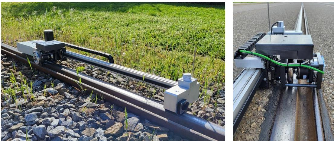
Fig. 22 BUT rail tribometer
