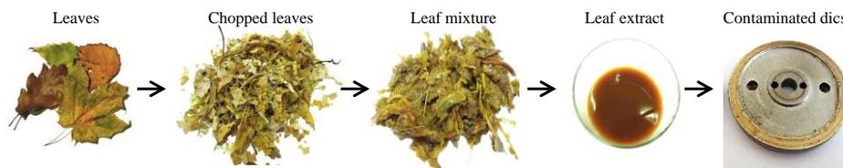
Fig. 7 Preparation of leaf-contaminated condition on test sample [63]
