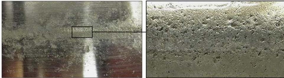
Fig. 11. Photographs of wheel disc surface after 300 cycles when sanding under wet conditions.
