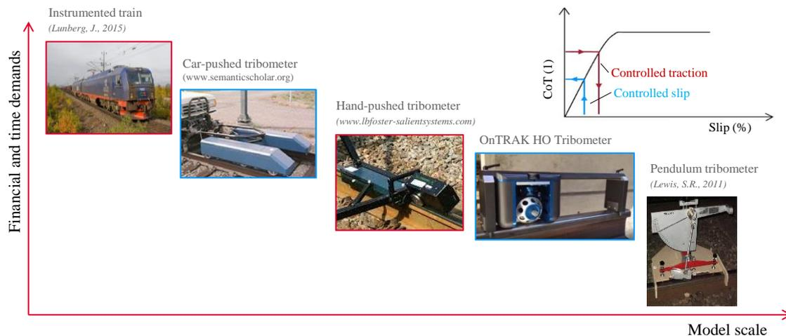
Fig. 18 Various approaches for field measurement of wheel-rail coefficient of adhesion.
