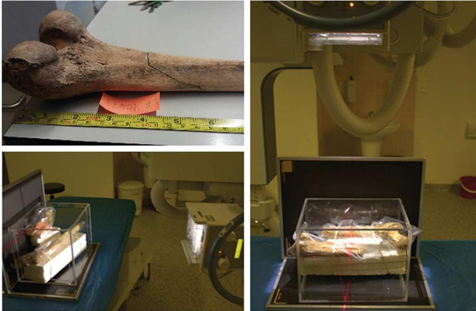
**Fig. 6.** Physically reduced dry cadaveric femur involved in the study (*top-left*), capturing an anterior-posterior radiograph of the experimental setup (*right*), taking a lateral radiograph (*bottom-left*).
