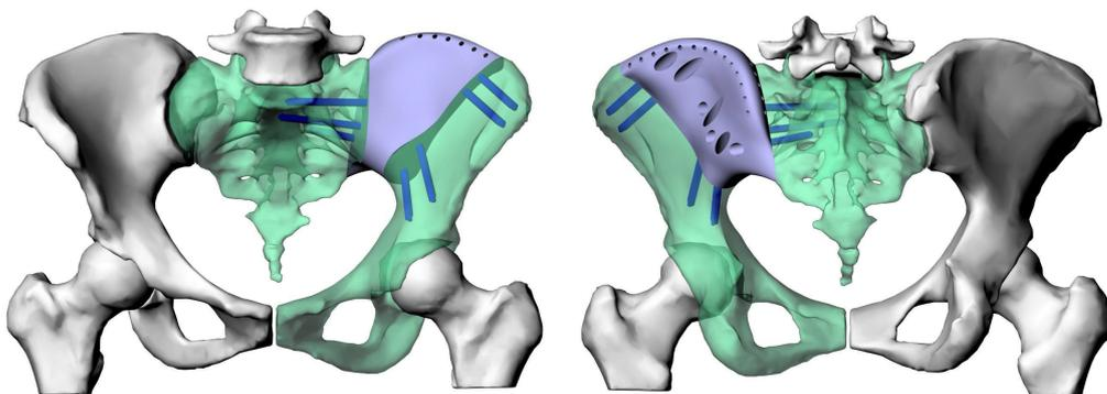
**Figure 2.4: Patient specific implant** designed on digital 3D anatomical models of the pelvis and hip joint from a CT scan. If the part of the anatomy replaced by the implant is more significant, and it is impossible to use mirroring of the healthy part of the anatomy, 3D shape modelling approaches learned on a large patient population greatly help in designing the suitable implant shape. Image courtesy of TecuMed, s.r.o.
