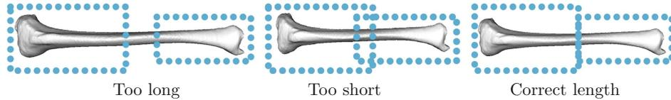
**Fig. 4.** Relation between vertex assignment and resulting bone length. No assignment of the vertices in the middle of the shaft to any of the fragments leads to a bone that is too long (*left*). Assignment of the vertices to both fragments results in a bone that is too short (*middle*). The correct length is ensured by assigning each vertex to exactly one fragment (*right*).
