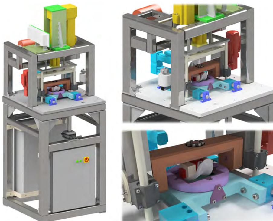
Fig. 2. Model of the test device with the detail of the contact couple and optical module.
