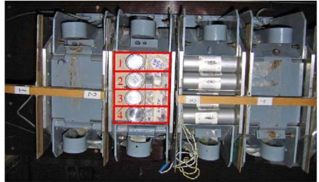
**Fig. 2.** Top view of the “Energy plus Transmutation” set-up with radioactive samples placed on top of it. Beam enters from the left side. The samples shown in this figure are assumed to occupy a volume of  $36 \times 36 \times 1.5 \text{ cm}^3$  for the sake of simulation by MCNPX.
