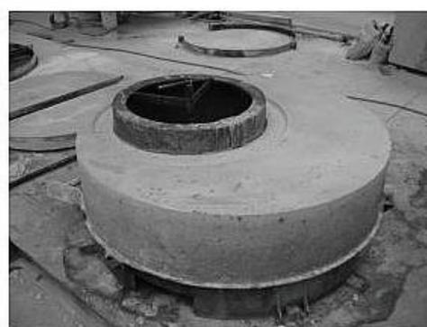
**Fig. 6.** Transition board made from geopolymer concrete
