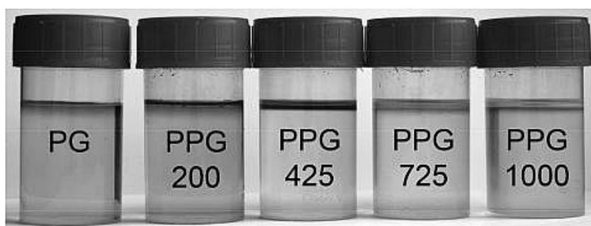
Fig. 3—Miscibility of surfactants in alkali activator solution (sodium waterglass).
