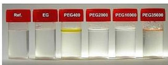
Fig. 9. Miscibility and color change of used glycols in activating solution of the same composition as for pastes with 2% addition of glycol after 14 days.
